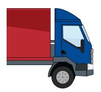
The Lorry with the shaped cab will have less air resistance. This lorry will use less fuel. It will cause less pollution and be cheaper to run.
